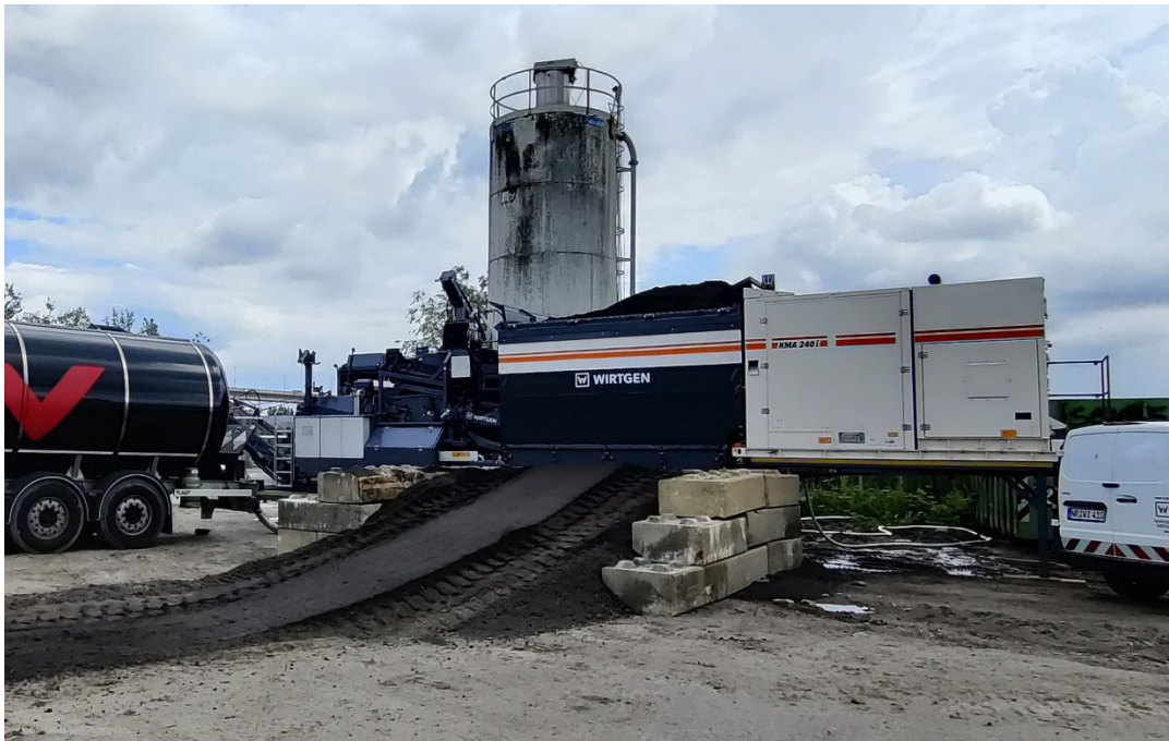
Figure 3. In-plant cold recycling (production)
