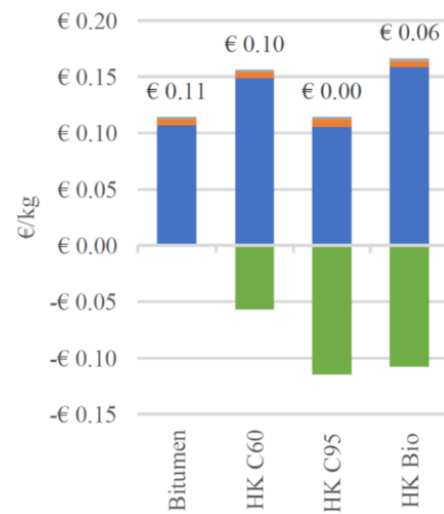
Figure 2. ECI of 60% biocircular (HK C60), 95% biocircular (HK C95) and
